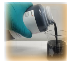
NMP dispersion for LIB cathodes
